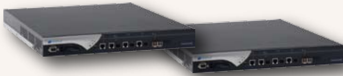
The central intelligence of highly available storage solutions is represented by both of the mirrored SANRAD 3400 switches
